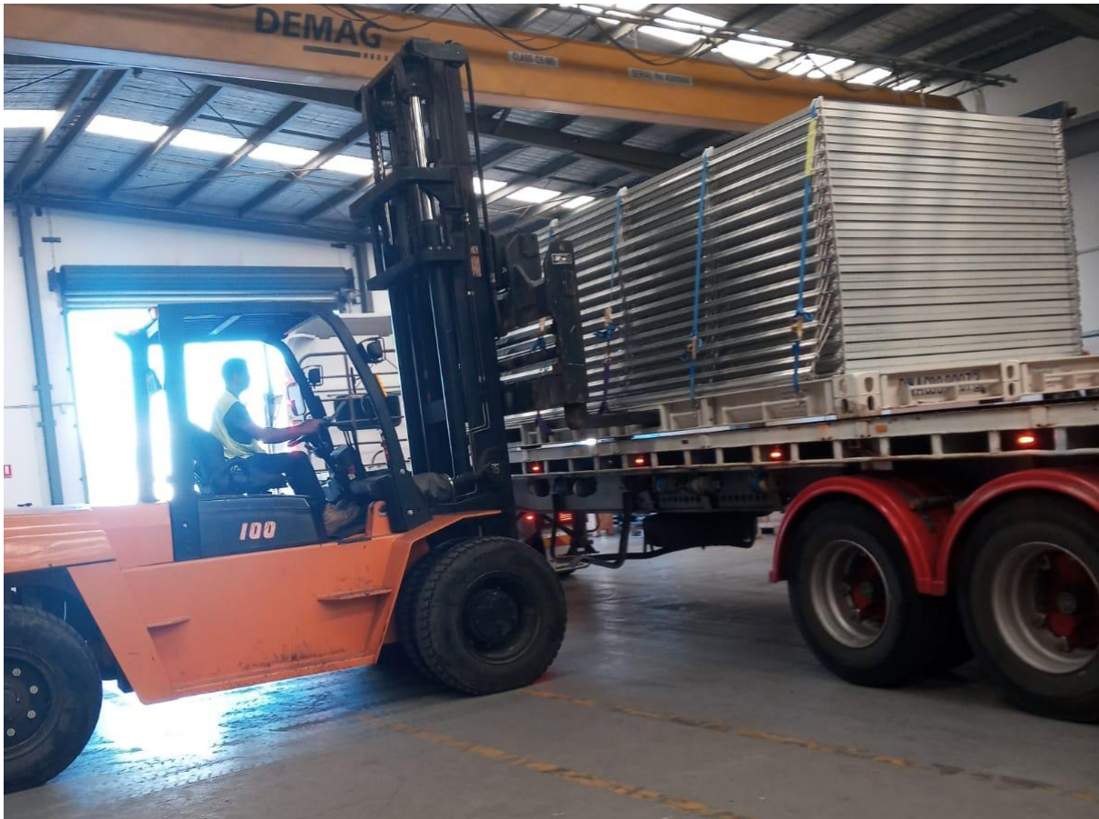
Example of lifting onto a flatbed using a 13 tonne forklift
