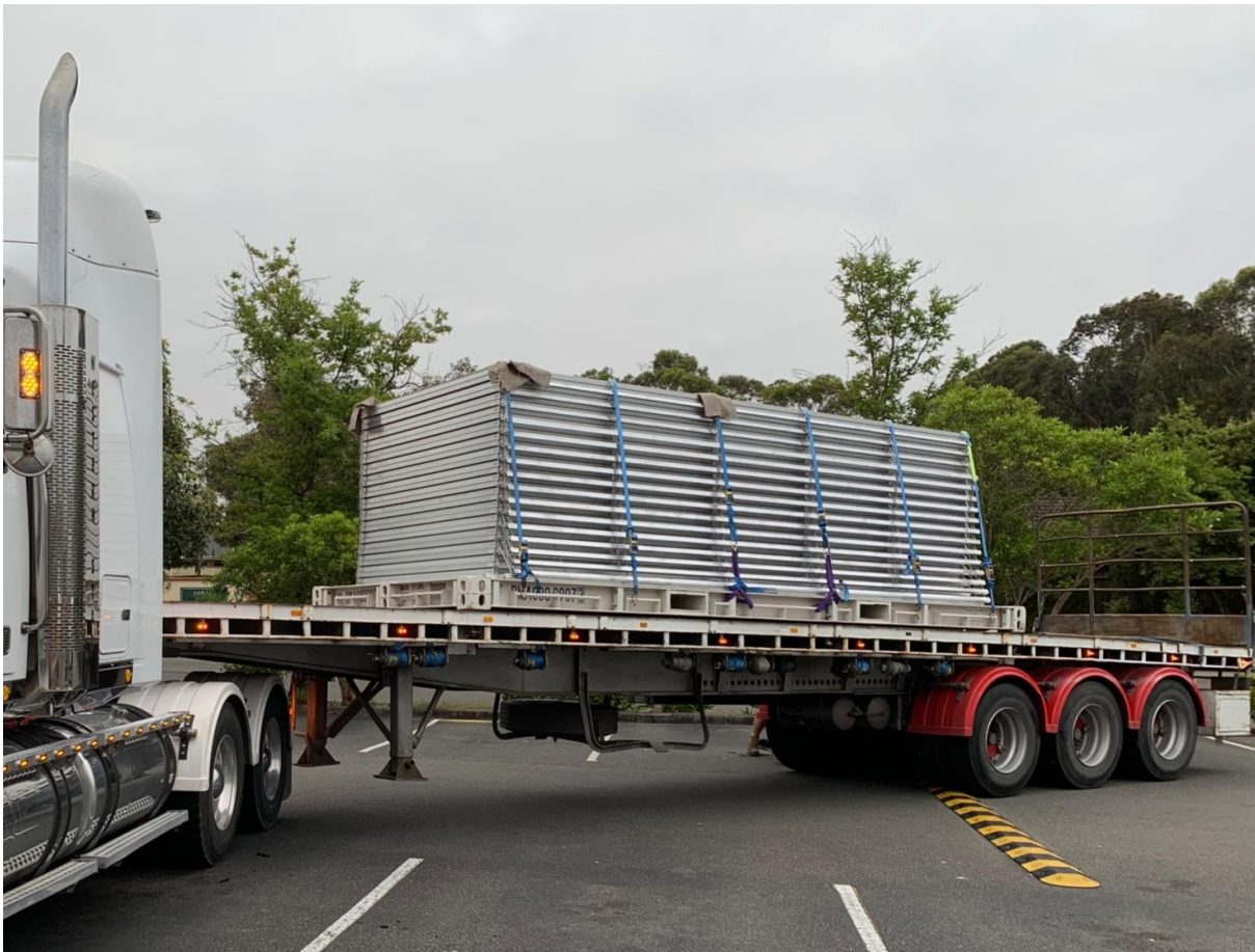
Example of a stack of Solpods on a pallet (container base) on a flatbed trailer, secured with twist-lock pins, prior to coverage with a heavy tarpaulin.
