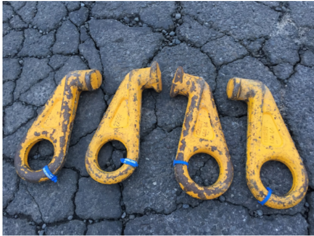
Lifting lugs to suit corner castings of container base.
