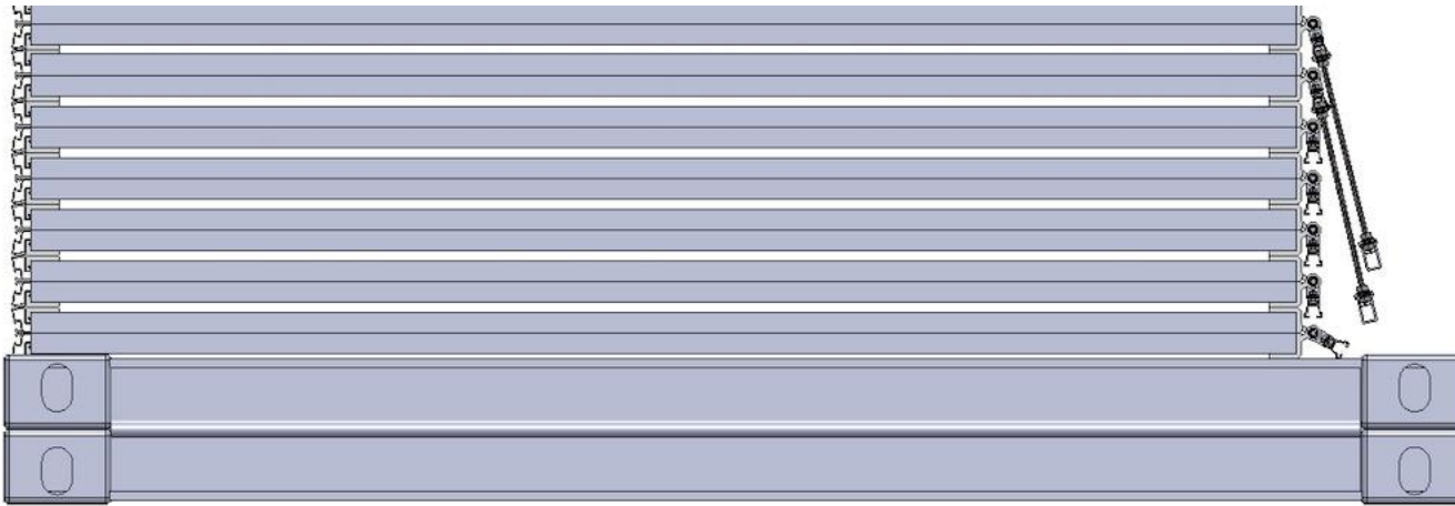
Side elevation of Solpod v4-S20-Tilt stacked on a container base Note that the spine legs and spine lower beam are missing from the bottom four units
