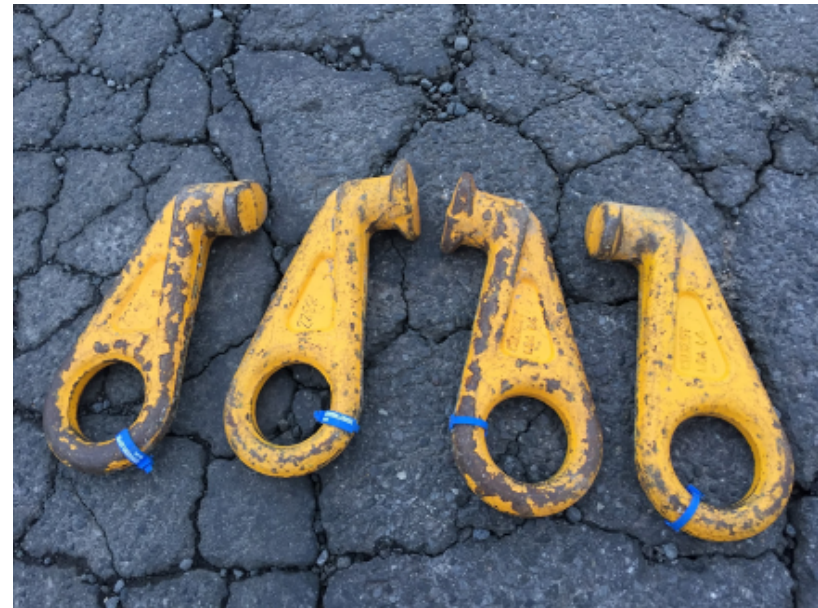
Lifting lugs to connect to corners of container base
