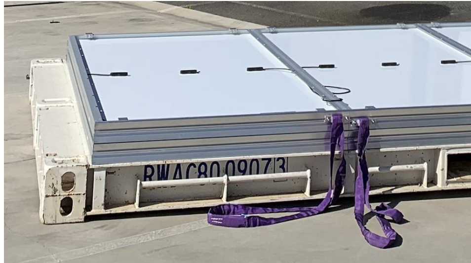
Sling brackets are offset Sling brackets are on on different edge beams (upper and lower)
