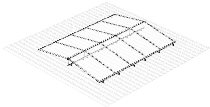
Solpod on 22 roof clamps (high wind regions)
